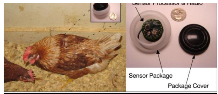
Fig: Photograph of a laying hen wearing a wireless sensor
