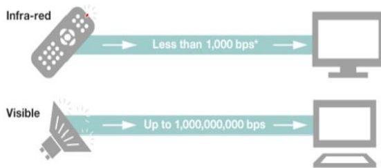
Figure 2. The operation principle of Li-Fi and TV remote control system [10] (*bits per second)
