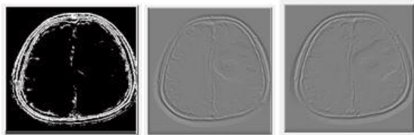
Fig 6: Edge detected output, Vertical gradient, Horizontal gradient
