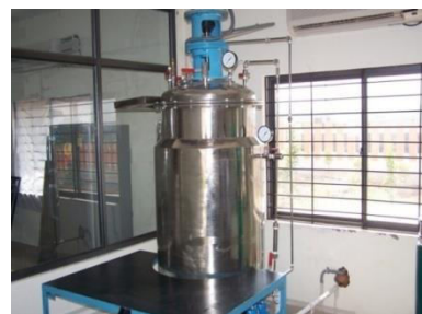
Fig-2: T. viride growth on PDA plate Fig-3: TSM and PDA flasks with T.viride growth Fig-4: Fermentor in the production unit
