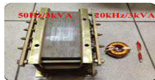
Fig. 1. Comparative photo of 50-Hz LF and 20-kHz HF transformers
