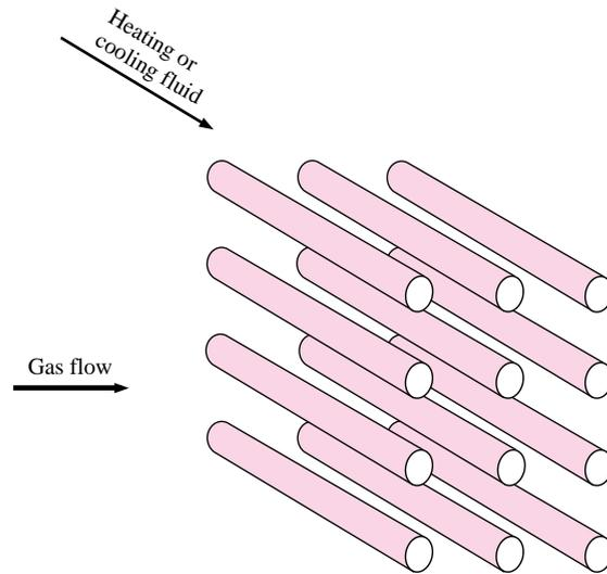
**Figure 10-5** | Cross-flow heat exchanger, both fluids unmixed.
