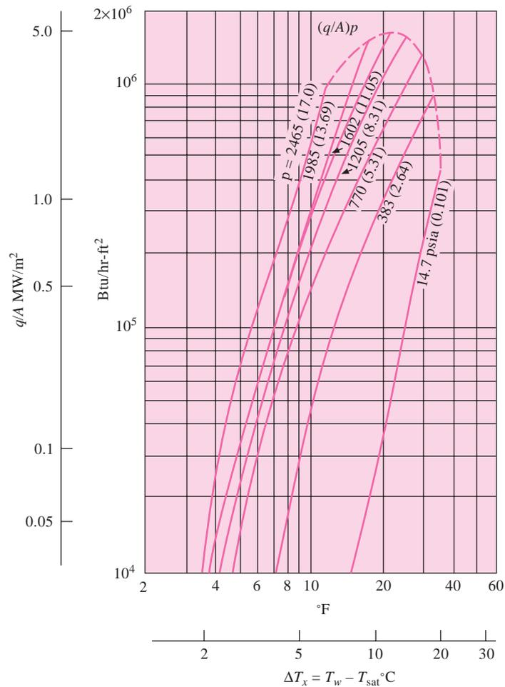
**Figure 9-9** | Correlation of pool-boiling data by Equation (9-33), from Rohsenow [5].
