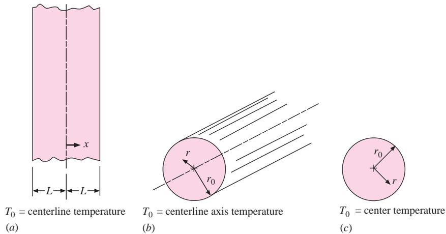
**Figure 4-7** | Midplane temperature for an infinite plate of thickness  $2L$ : (a) full scale.
