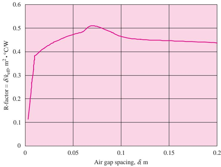
**Figure 12-17** | Free convection across horizontal air gap heated from below at 300 K. See Equation (7-64) and Table 7-3.
