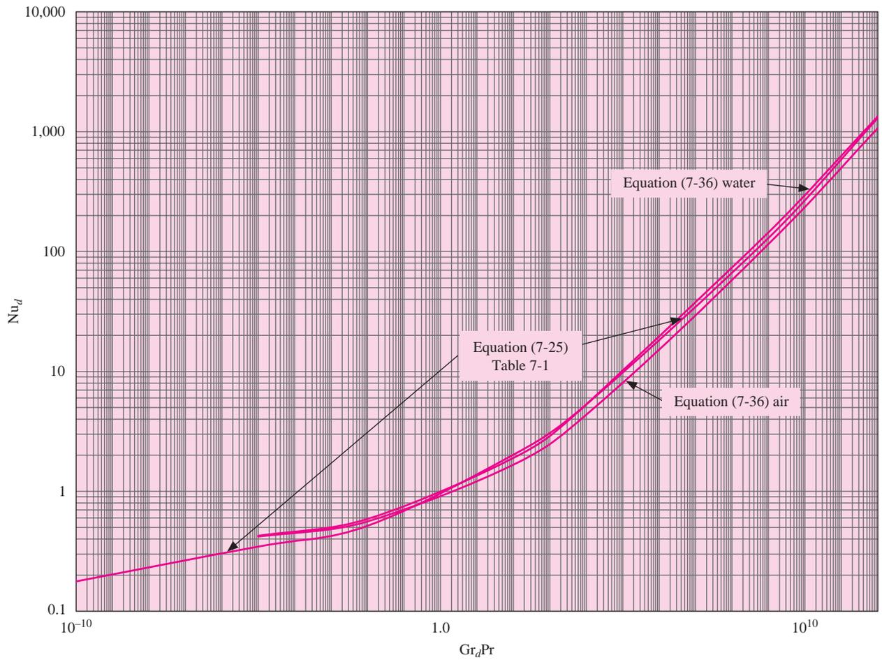
**Figure 12-10** | Nusselt numbers for free convection from isothermal spheres. Properties evaluated at film temperature  $T_f = (T_w + T_\infty)/2$ .
