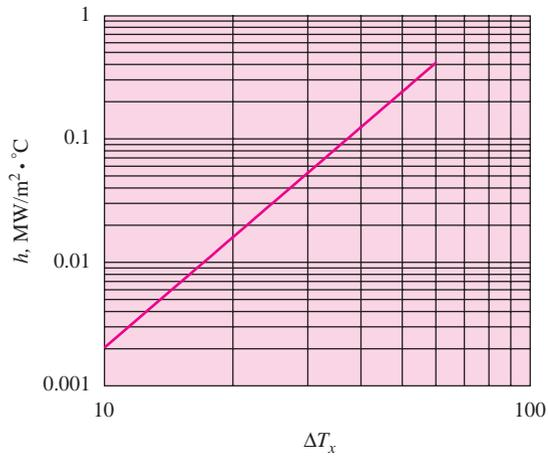
**Figure 12-24** | Approximate boiling heat-transfer coefficients for water at higher pressures ( $0.7 < p < 14$  MPa). See Equation (9-36).
