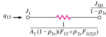
**Figure 8-54** | Complete radiation network for system in Figure 8-51.
