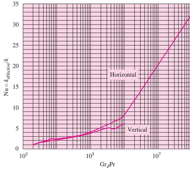
**Figure 12-16** |  $R$ -factor for free convection across vertical air gap at 1 atm pressure, 300 K,  $\Delta T = 10$  K,  $L = 0.2$  m. See Equation (7-64) and Table 7-3.
