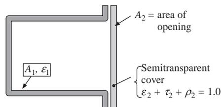
**Figure 8-60** | Radiation network for cavity with partially transparent cover.
