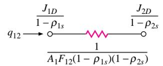
**Figure 8-48** | System with one specular-diffuse surface.
