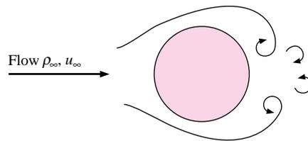
**Figure 6-8** | Velocity distributions indicating flow separation on a cylinder in cross flow.
