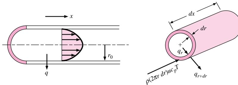
**Figure 5-16** | Force balance on fluid element in tube flow.
