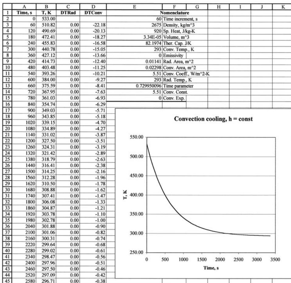
The resulting cooling curve is plotted in Figure Example D-6(b) along with a few rows of the calculations. Note that the temperature decrements due to radiation and convection are about the same at the start of cooling; thus, to neglect radiation would produce a serious error.
