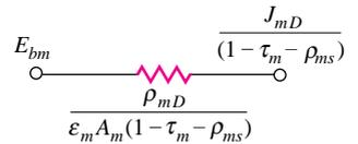
**Figure 8-57** | Complete radiation network for system in Figure 8-55.
