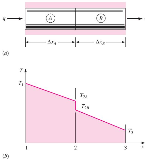
**Figure 2-16** | Joint-roughness model for analysis of thermal contact resistance.
