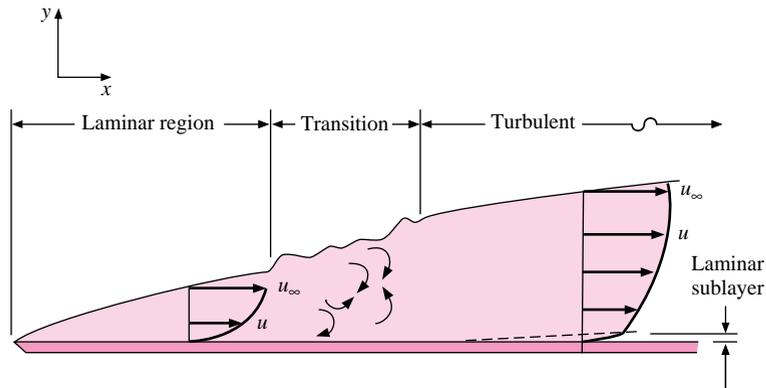
**Figure 5-2** | Laminar velocity profile on a flat plate.
