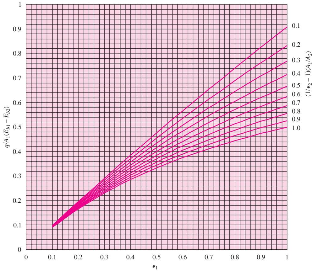
**Figure 12-21** | Radiation heat-transfer coefficient for a blackbody in a large enclosure at 300 K. See Equation (8-115). Note:
