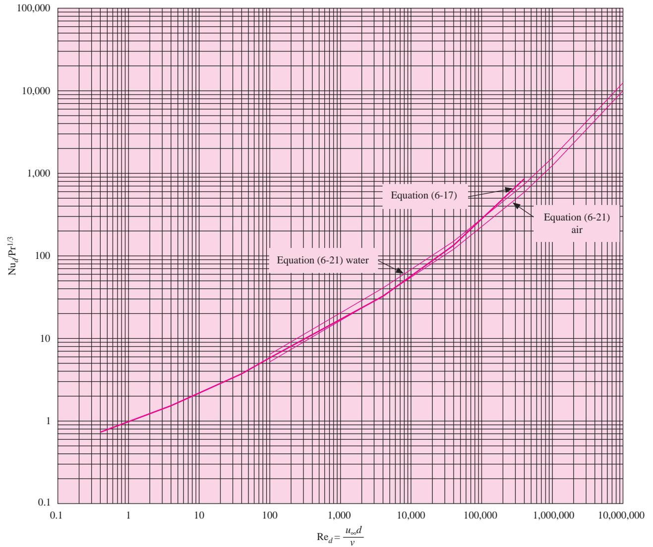
**Figure 12-7** | Nusselt numbers for cross flow over isothermal spheres. Properties evaluated at free-stream temperature  $T_\infty$ , except  $\mu_w$ .
