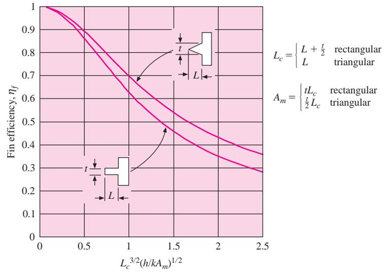
**Figure 2-12** | Efficiencies of circumferential fins of rectangular profile, according to Reference 3.
