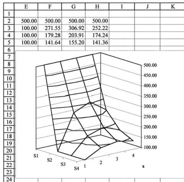
Plate with Boundary Heat Source and Convection
