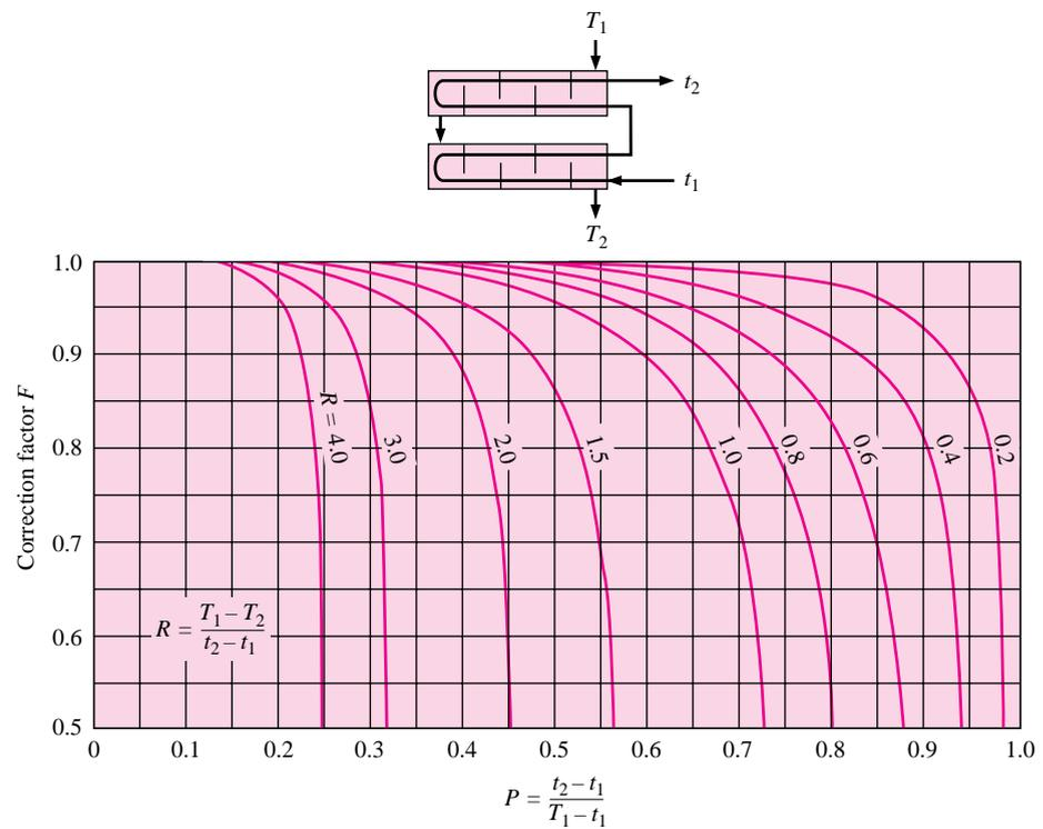
**Figure 10-10** | Correction-factor plot for single-pass cross-flow exchanger, both fluids unmixed.
