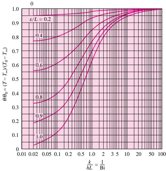
**Figure 4-11** | Temperature as a function of axis temperature in an infinite cylinder of radius  $r_0$ , from Reference 2.
