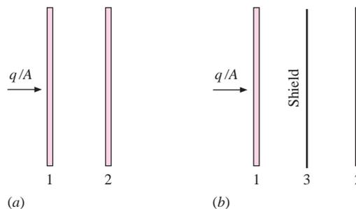
**Figure 8-34** | Radiation network for two parallel planes separated by one radiation shield.
