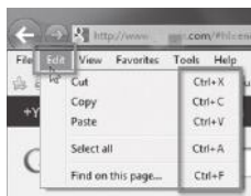
Figure 1.6 An interface providing both menus (for novice users) and hot keys (for expert users).
