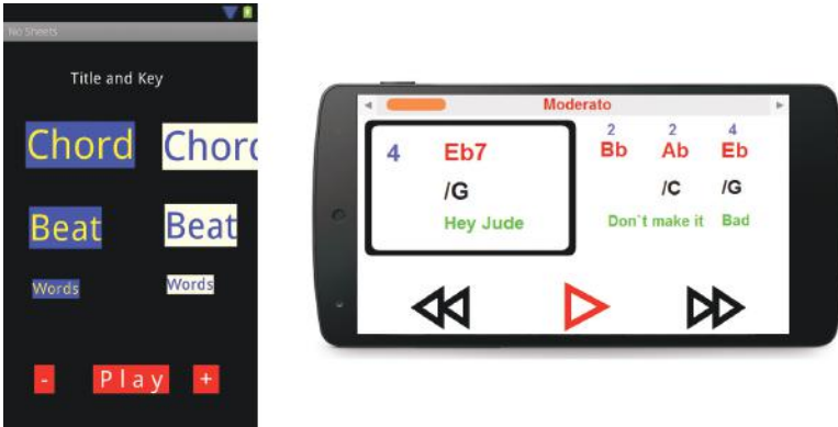
Figure 8.6 The initial (left) and redesigned (right) “play” activity/layer for No Sheets: The new design after evaluation uses a landscape mode and fewer primary colors. The icons for fast-forward and review are changed to the conventional style, and the current tempo is shown on top.
