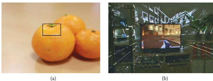
Figure 3.8 (a) An ideal display that would provide relatively higher resolution in the area of the user's focus; (b) a large immersive display as realized by a high-resolution monitor in the middle- and lower-resolution projection in the periphery. (From Microsoft® Research, CHI 2013: An Immersive Event (Illusions create an immersive experience), 2013, http://research.microsoft.com/en-us/news/features/chi2013-042913.aspx [9].)
