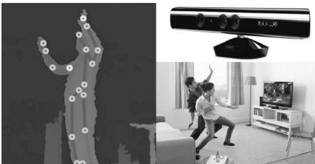
Figure 9.6 Whole-body skeletal tracking using the Kinect depth sensor (left) and its application to motion-based games (right).
