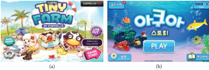
Figure 2.6 Comparison of two mobile game interfaces (the initial entry screen): (a) information and object density is needlessly high and distracting (left), (b) simple and minimal layout, and object sizes fitted to ergonomic usage (right). (From http://www.withhive.com .)
