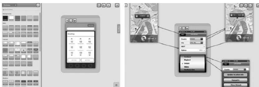
Figure 4.16 An example of a wire-framing tool (FluidUI, https://www.fluidui.com ). Designing the content of a screen (left) and overall interaction behavior, e.g., how screens switch upon interaction (right).
