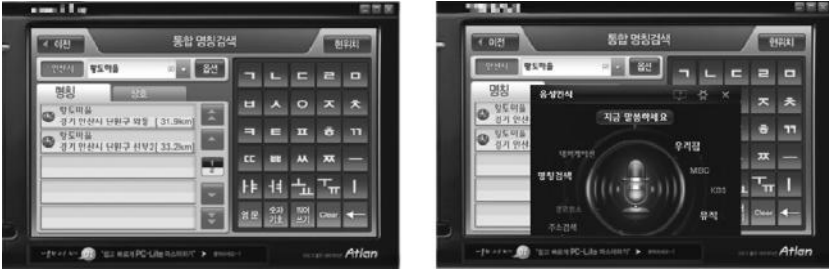
Figure 9.15 Alternative multimodal interfaces in the vehicle navigation systems (touch and voice). (From Finedrive, http://www.fine-drive.com .)
