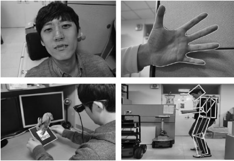
Figure 9.5 Camera-based motion-tracking examples (for face, hand, marker, and whole body).
