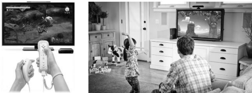
Figure 9.14 Multimodal interaction in games (left) using the buttons for setting selection, and (right) action gestures for the game play itself (Microsoft Kinect, http://www.xbox.com/en-us/kinect ; Nintendo® Wii, http://www.nintendo.com/wii/features ).
