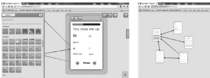
Figure 4.26 Initial design wireframe for No Sheets 1.0 using a wire-framing tool. Left: Icons and GUI elements in the menu in the left can be dragged onto the right to design the interface layer. Right: Navigation among the design layers can be defined as well (indicated by the arrows).
