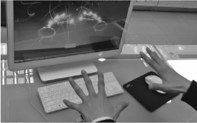
Figure 9.9 Finger-based interaction using the Leap Motion. (From Leap Motion, Leap Motion Controller, 2014, http://www.leapmotion.com [7]).
