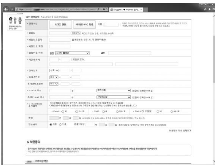
Figure 2.4 Display layout and user interfaces for facilitated date entry: Selection menus, default values, and structured forms are used to reduce errors. (From Smith, S. L., and Mosier, J. N., Guidelines for Designing User Interface Software , Mitre Corporation, Bedford, MA, 1986 [4].)
