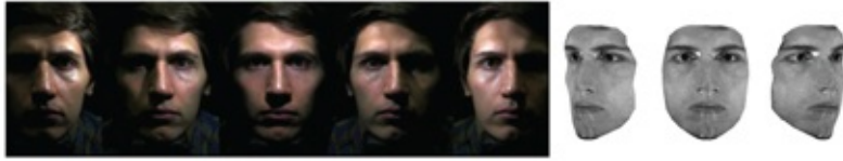
Figure 11.22 . This figure shows the results of photometric stereo on color images in the presence of shadows. On the left we see the input images and on the right the reconstructed face geometry is shown from different views.
