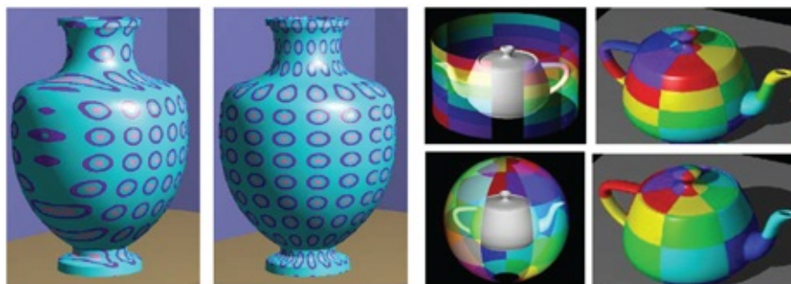
Figure 14.12 This figure shows orthogonal (left) and cylindrical (right) mapping on a vase and a cylindrical mapping (top) and a spherical mapping (bottom) on a teapot.
