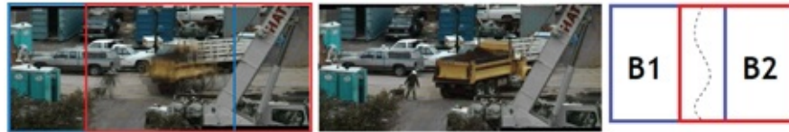
Figure 11.17 . On the left you see two images (shown by red and blue rectangle) with a large overlap in between that are composited using blending. Since the people and the truck moved between the capture of these two images, this results in severe ghosting of the moving objects. On the right, the same two images are composited using an image cut operation resulting in a artifact free composition.
