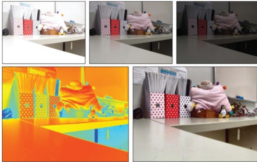
Figure 10.13 .Top Row: Three different images captured at different shutter speeds. Bottom Left: The recovered high dynamic range radiance map. Note that this image cannot be displayed in the regular display since it has a much higher contrast. Therefore we show a heat map visualization of the radiance, blue indicating low and red indicating high. Right bottom: This shows the same image being shown on a regular 8-bit display using a tone-mapping operator.
