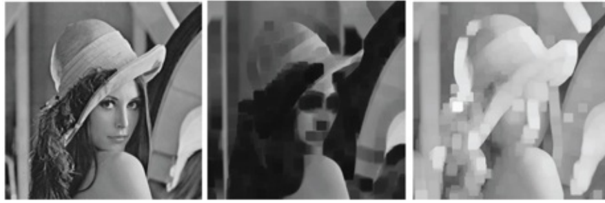
Figure 5.28 . This figure illustrates the effect of the minimum (middle) and maximum (right) filter on an image (left) to achieve the effects of erosion and dilation respectively.
