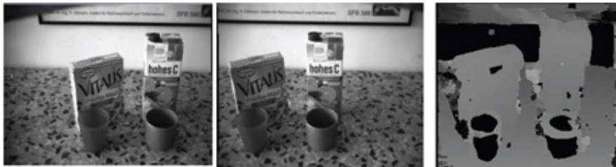
Figure 8.9 .This image shows two rectified images (on left) and the depth reconstructed from them (on right).
