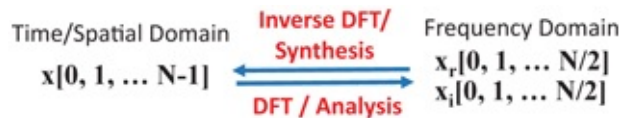
Figure 4.2 . This figure shows the processes of DFT and inverse DFT converting a signal in time/spatial domain to its representation in frequency domain and viceversa.
