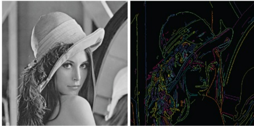
Figure 5.19 . The figure shows the effect of local edge aggregation. Left: The original image; Right: The image with edgels detected by Canny edge detector which are then linked by local aggregation. Each linked edge is colored with a different color, not necessarily unique.
