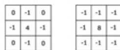
Figure 5.12 . The Laplacian operator considering only four perpendicular neighbors (left) and considering all eight neighbors (right).
