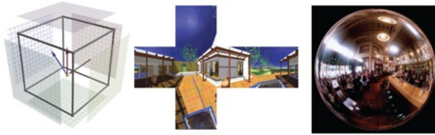
Figure 14.22 This shows a cubic and spherical environment map. The cubic map is shown unfolded (middle) and is generated by using a 6-pass rendering each rendering a face of a cube (left) seen from the center of the cube. The spherical map (right) is generated from images of a cafe taken using a fish-eye lens camera.
