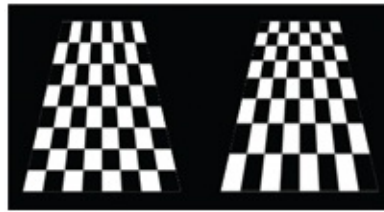
Figure 14.13 A texture mapped polygon with depth going from the front to back. The texture coordinate assignment on the left does not account for perspective projection and therefore the shrinkage of the checkerboard squares is only in the horizontal direction due to the trapezoidal shape of the polygon. The size squares of the checkerboard on the right change based on the depth due to the perspective correct texture coordinate assignment.
