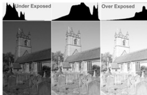
Figure 11.2 . This figure shows how the exposure (the measure of how much light is let into the camera to capture the picture) affects the histogram of an image. When the image is underexposed (left) the histogram h shifts left with higher values of h for lower values of i . When the image is overexposed (right) the histogram h shifts right. For correctly exposed image, the values of h at 0 and 255 are not outliers.
