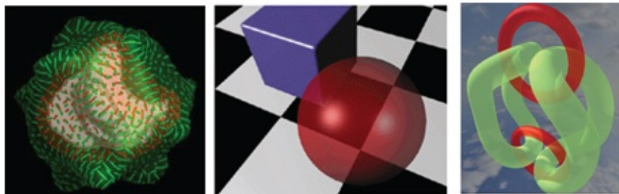
Figure 14.26 The figure shows rendering of transparency using alpha blending. Additional effects of lighting, shadows and texture mapping are included in the renderings.
