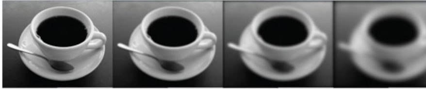
Figure 3.11 This image shows the effect of increasing the size of the box filter and convolving it with an image. From left: Original image and the same image convolved with a 3 \times 3 , 5 \times 5 and 15 \times 15 box filter.
