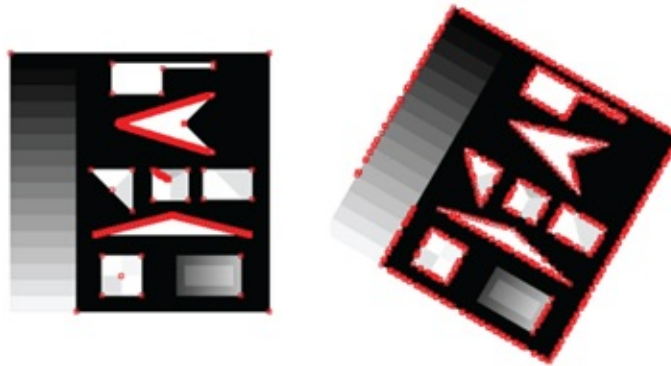
Figure 5.24 . This shows the features detected by the Morovac filter (in red) as the image orientation is changed by rotating it by 30 degrees. Vastly different pixels are now detected as corners.
